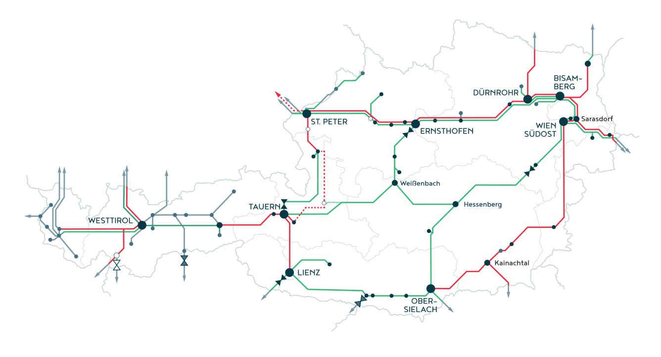
2,577 km — 380-kV line / under construction 9 APG grid node 3 M Phase-shifting transformer Power Grid
