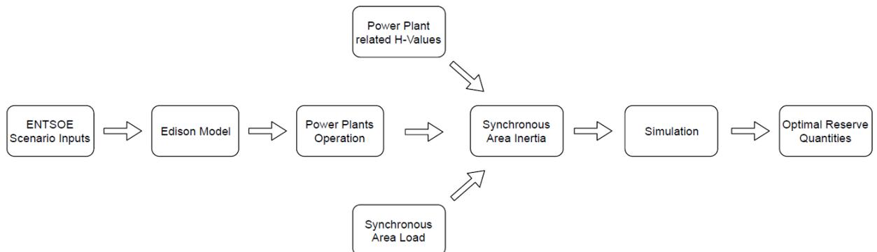
**Figure 71: Analysis flow for determining the optimal reserve quantities**
