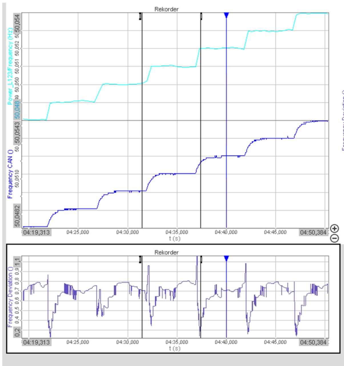
**Figure 49: Frequency deviation during frequency changes**
