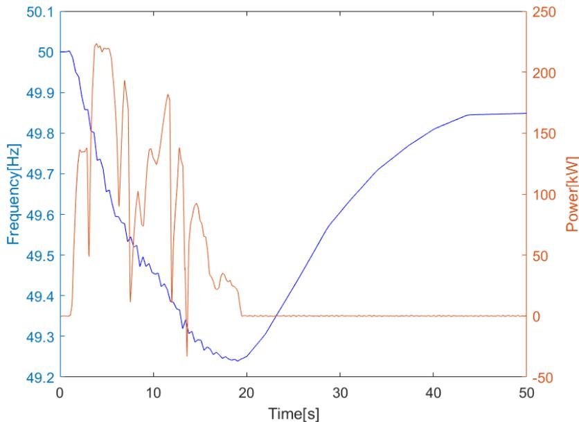
**Figure 42: SI under a slow frequency deviation (test III), under low frequency noise**
