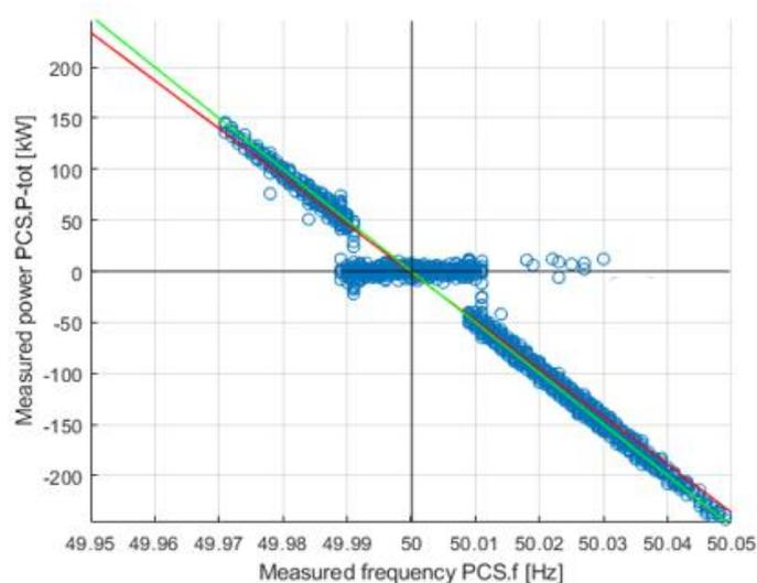
Figure 83: Check of the slope of FCR+ in the course of the field tests (Deadband = 10 mHz)
