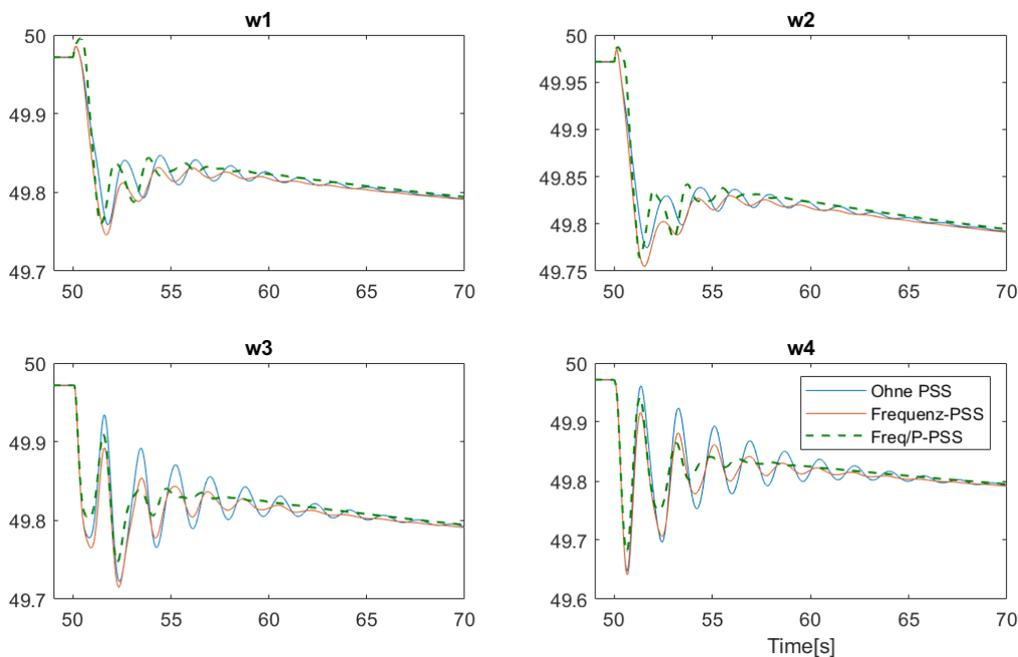
Figure 52 shows the decrease in performance when PSS only utilizes the frequency. Notice that in both cases (using frequency and power, or using only frequency) the same parameters
