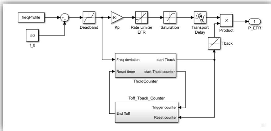
**Figure 28: Block description of the EFR function**
