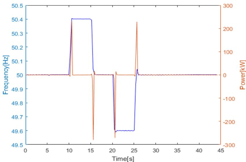
**Figure 39: SI function under a frequency step (test III)**
