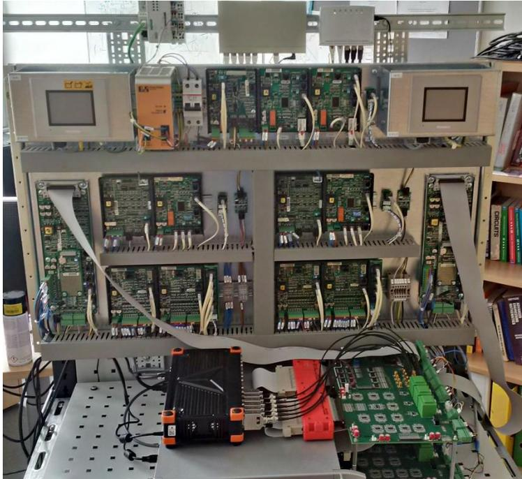
**Figure 27: C-HiL Setup with real-time simulator and control cards**
