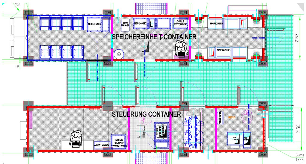
Figure 59: Layout of the energy storage system
