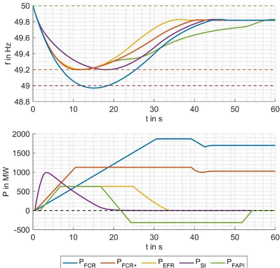
**Figure 13: Frequency and power curves for the investigated Frequency-Control-services**
