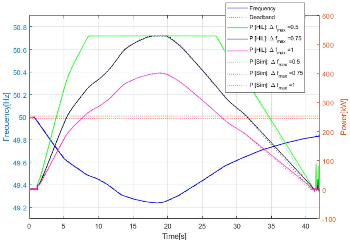
**Figure 30: Comparison of system response against expected response for different values of droop gains ( $\Delta f_{\max}$ )**
