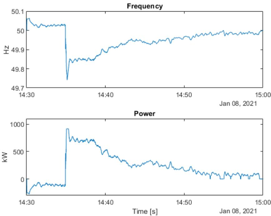
Figure 54 - Behaviour of EFR for a grid split event (Thold = 1800s)
