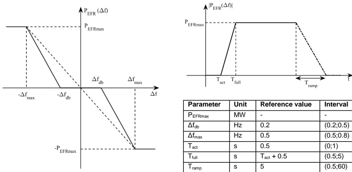
**Figure 8: Frequency- and time-characteristic curves of EFR**
