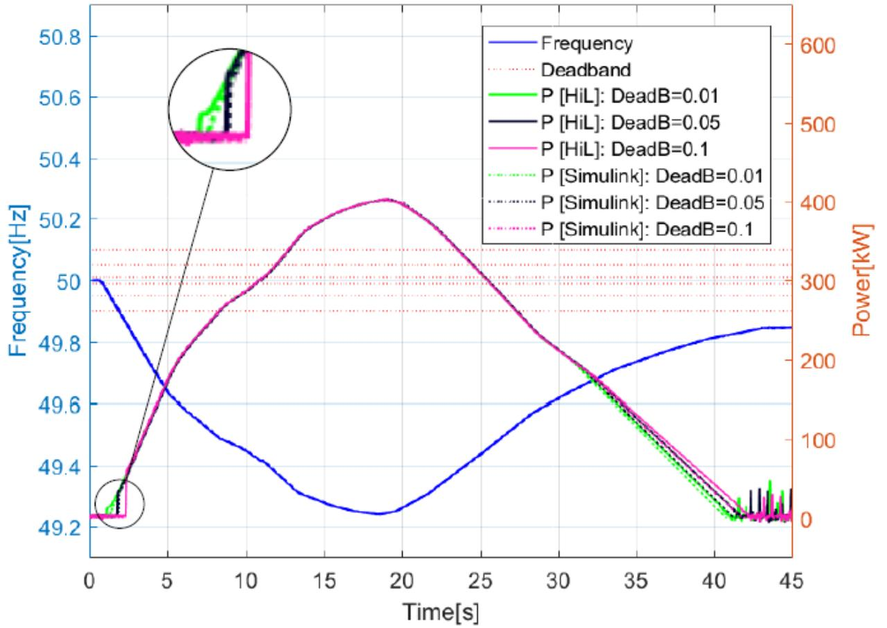
Figure 29: Comparison of system response against expected response for different values of deadband
