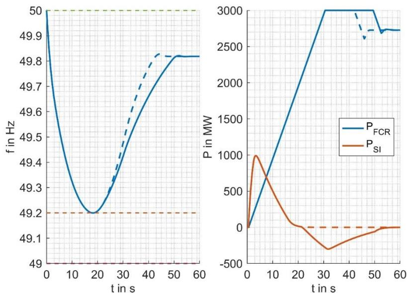
Figure 11: Frequency- and power-curves for SI
