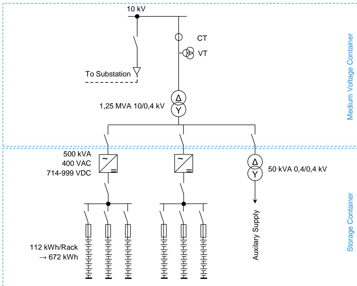
**Figure 58: Single Line Diagram of the ABS4TSO system**
