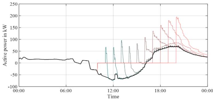
**Figure 25: PSR model aggregation for a 4-hour power interruption without BESS details [14].**
