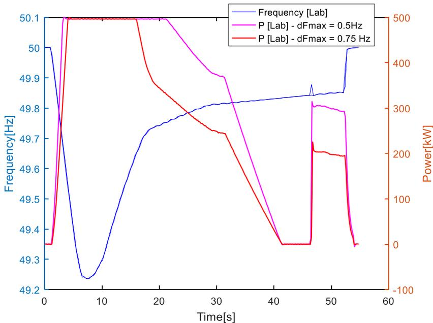
Figure 36: Effect of the droop parameter in the EFR response
