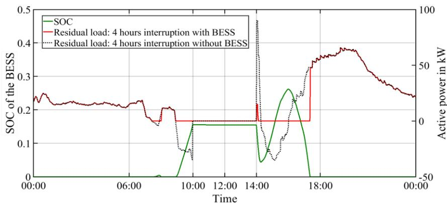
**Figure 24: PSR model aggregation for a 4-hour power interruption with BESS details [14]**
