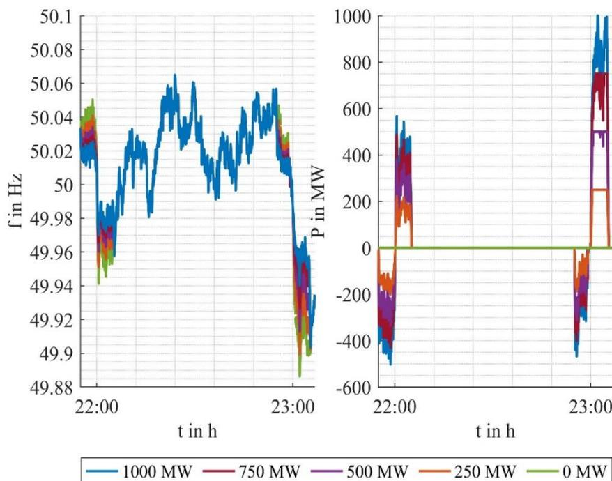
**Figure 22: Effect of a frequency-control-service against DFDs**
