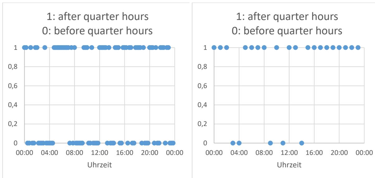
**Figure 21: Time distribution of maximal frequency deviations**
