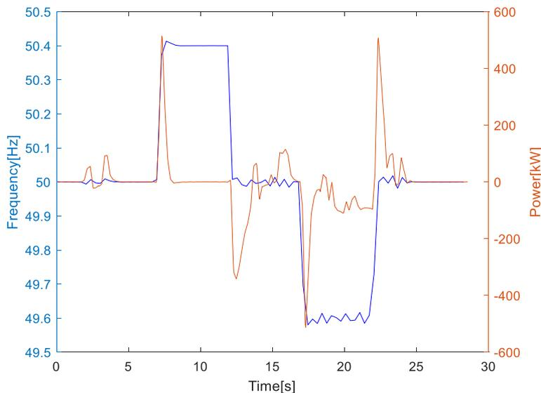
**Figure 37: SI function under a frequency step (test I)**
