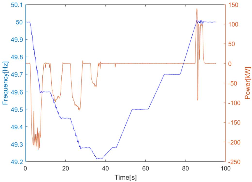
Figure 44: SI function for a synthetic frequency profile (test I)
