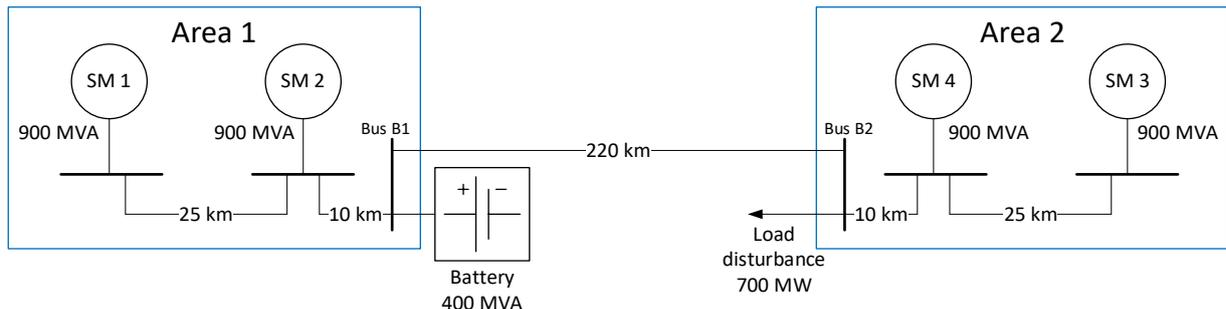
**Figure 15: Single-line diagram of the power system model**
