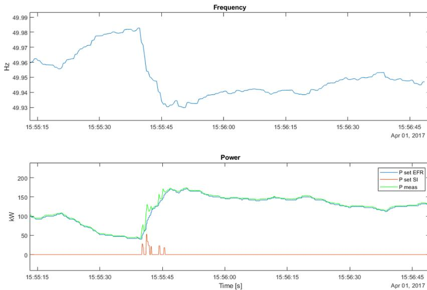
**Figure 57 - Behaviour of EFR + SI during multimodal operation**
