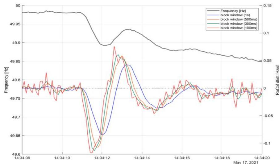
**Figure 82: Comparison of different sizes of the block window**
