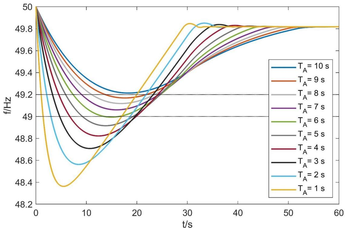
**Figure 6: Frequency curves following a reference incident for different values of  $T_A$**
