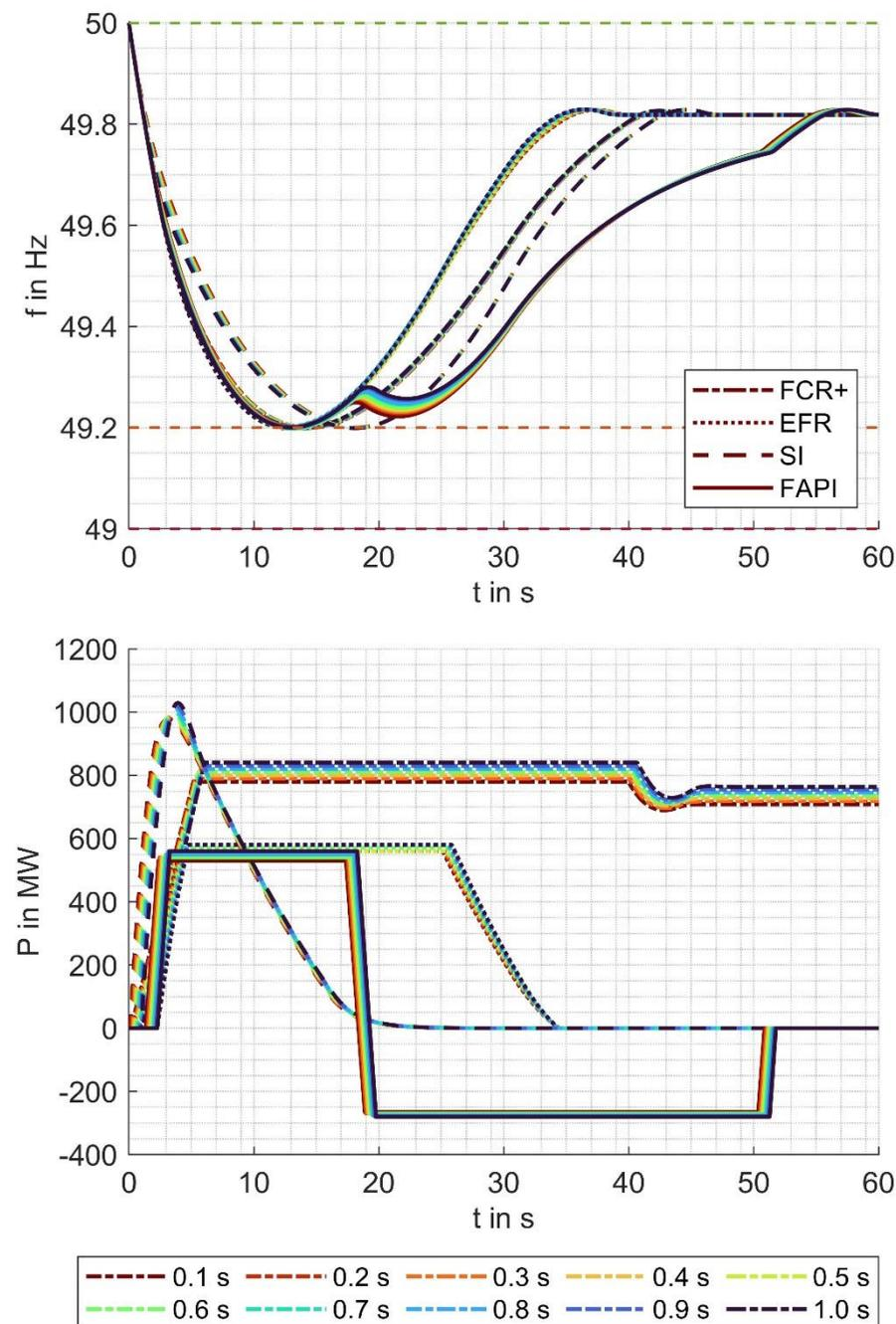
**Figure 14: Impact of the frequency measurement time on the effectiveness of the investigated frequency-control-services**
