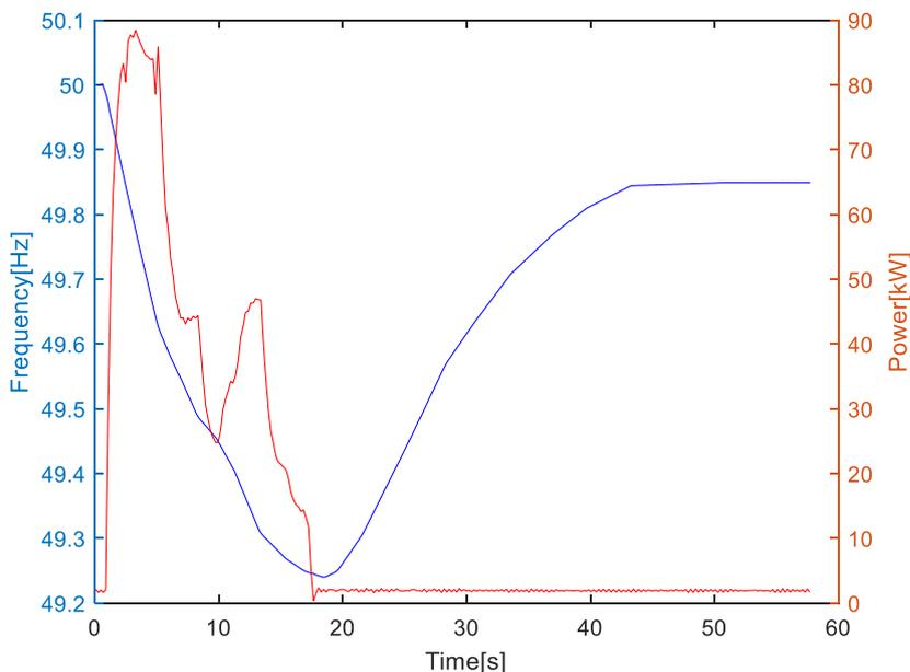
Figure 40: SI function under a slow frequency deviation (test I)
