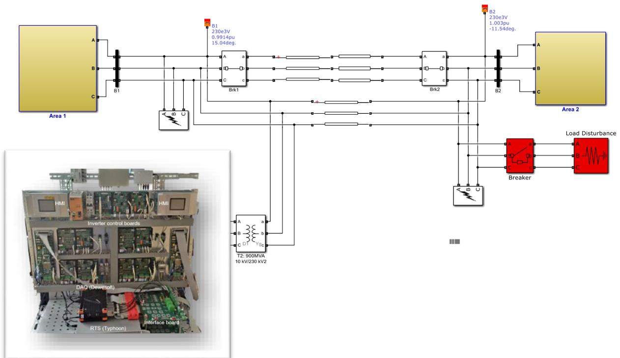
Figure 50: Two-Area network for PSS testing
