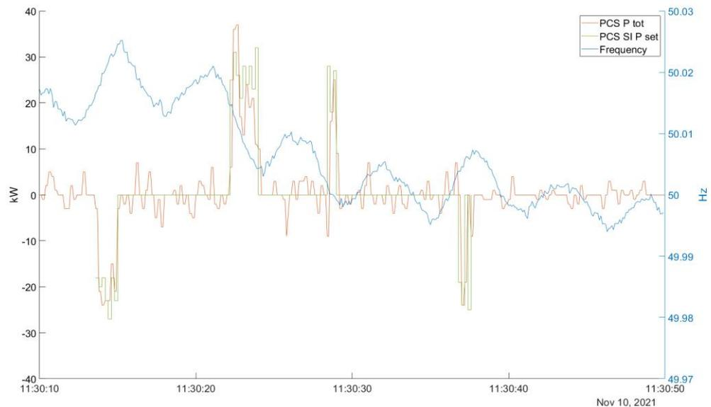
**Figure 67: Behaviour of SI under low frequency oscillations**
