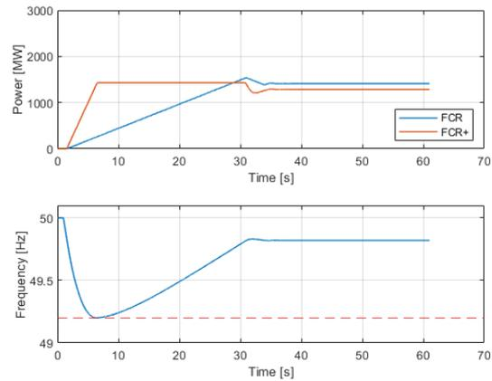
**Figure 81: Design hypothesis 2040 including FCR+ to keep the frequency  $\geq 49,2$  Hz**
