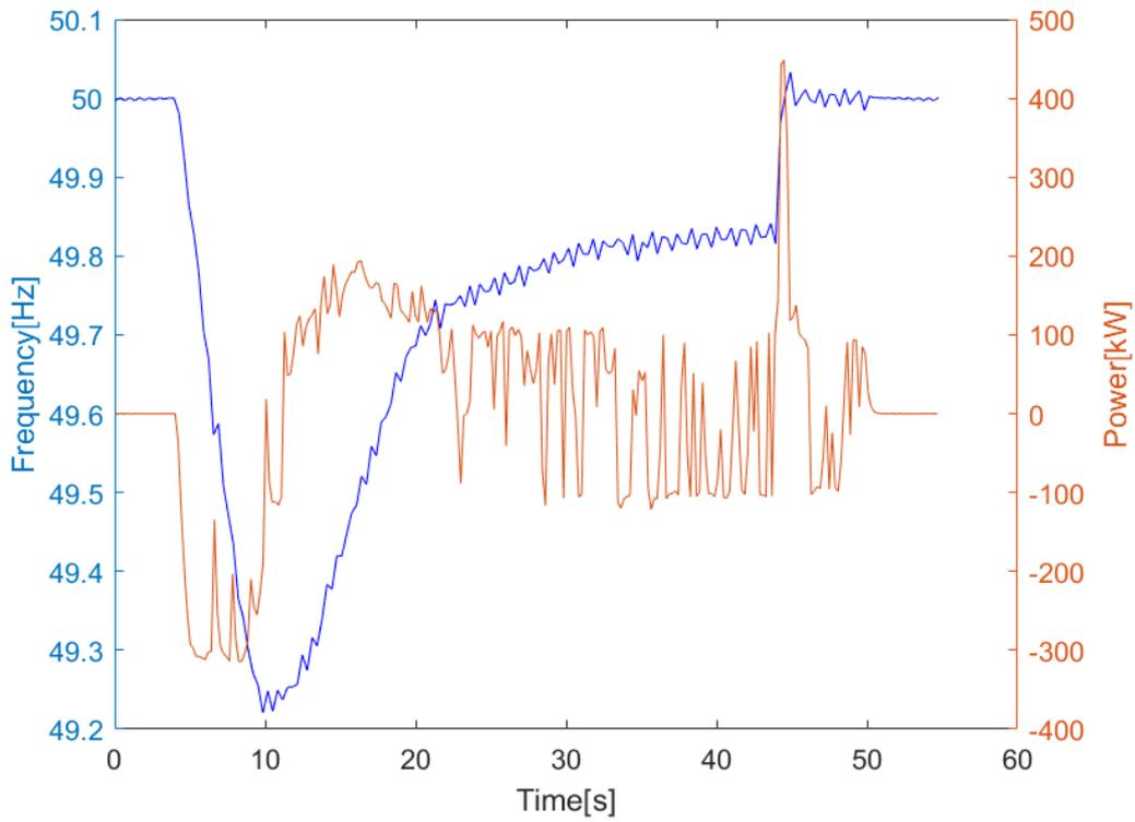
Figure 43: SI function under a large frequency deviation (with noise)
