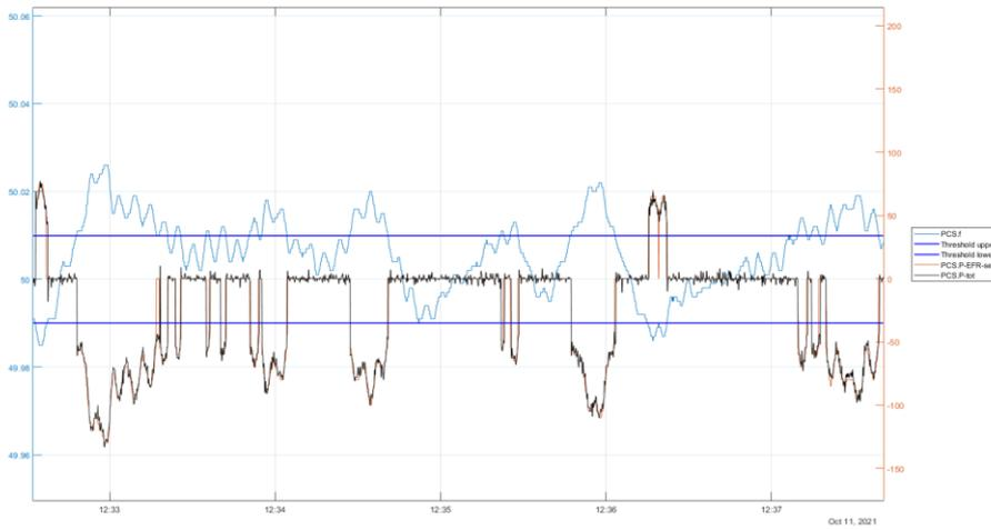
Figure 64: Behaviour of FCR+ with a deadband of 10mHz
