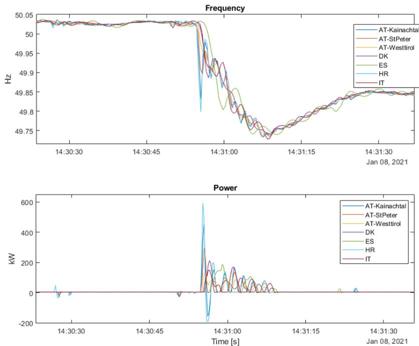
Figure 55 - Behaviour of SI for a grid split event using different frequency measurements (West region)
