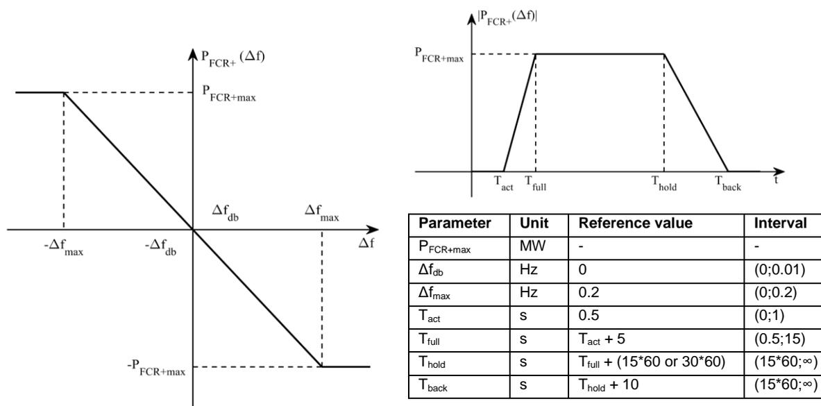
**Figure 7: Frequency- and time-characteristic curves of FCR+**
