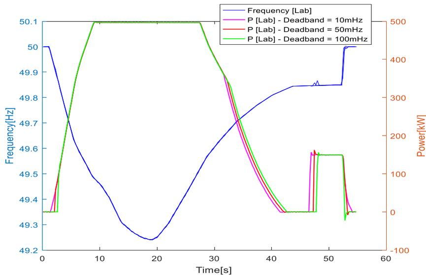
Figure 35: Effect of the deadband parameter in the EFR response
