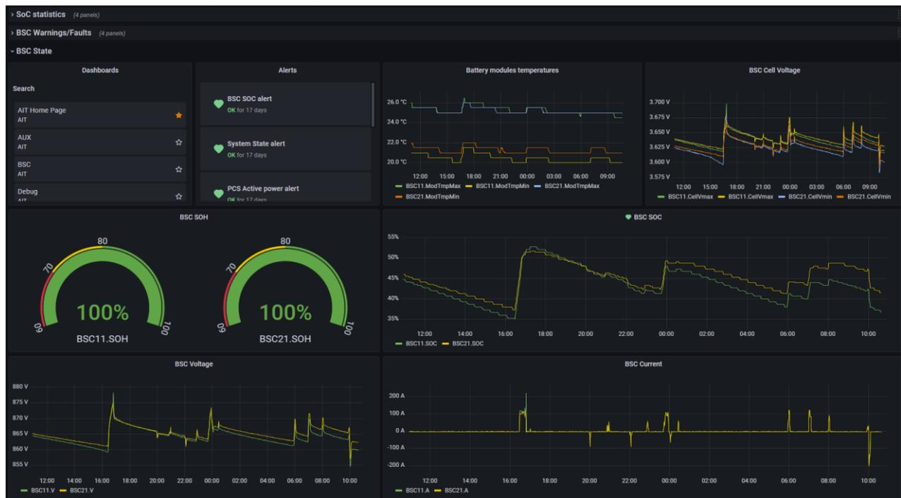
Figure 63: Screenshot of the graphical user interface to monitor the storage unit
