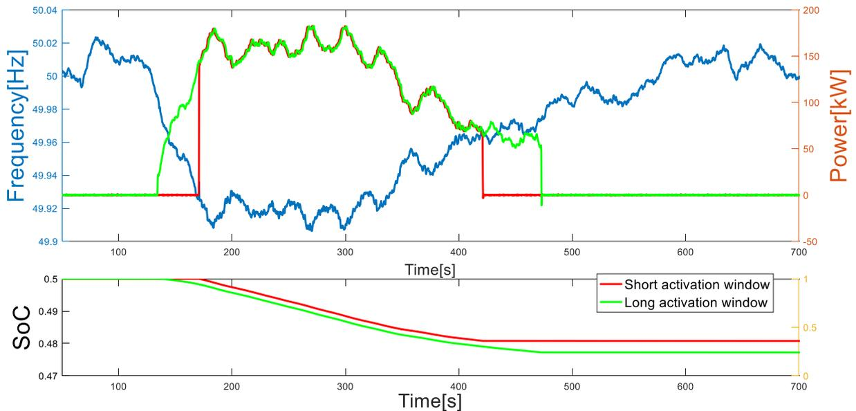
Figure 46: DFD response for two different activation windows
