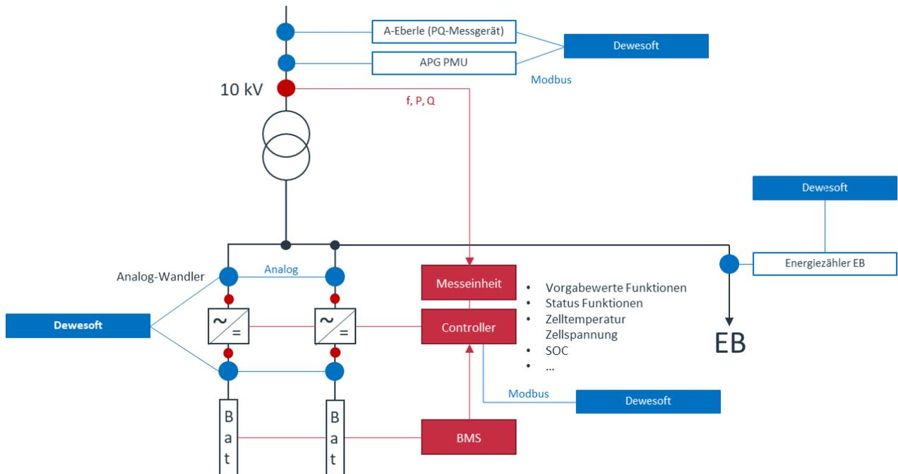
Figure 62: Measurement concept for the battery storage
