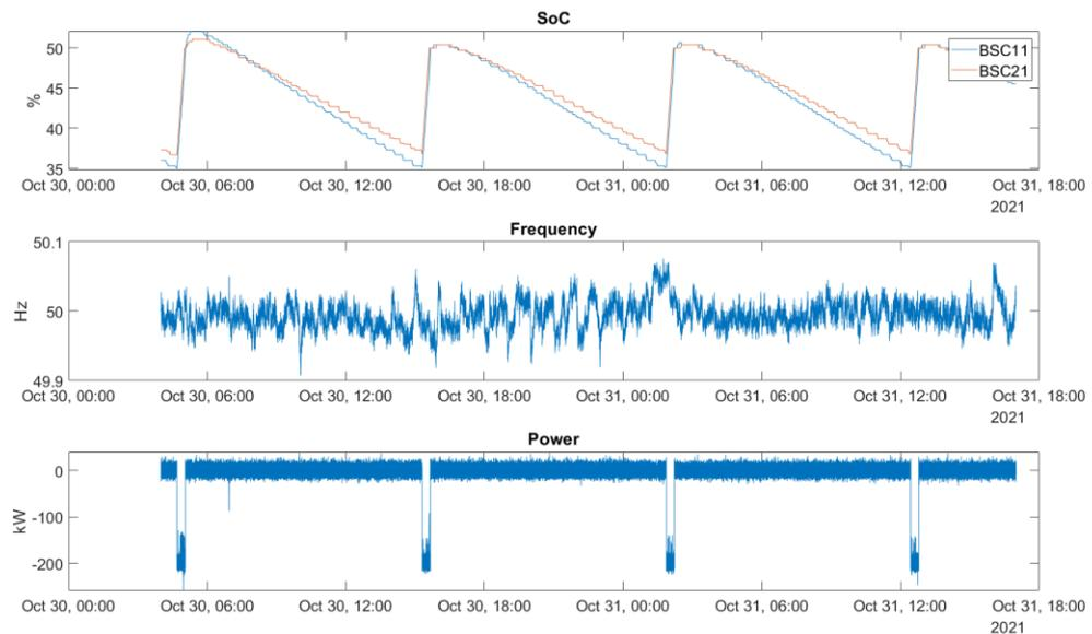
**Figure 68: Evolution of SoC under SI and no major frequency deviations**
