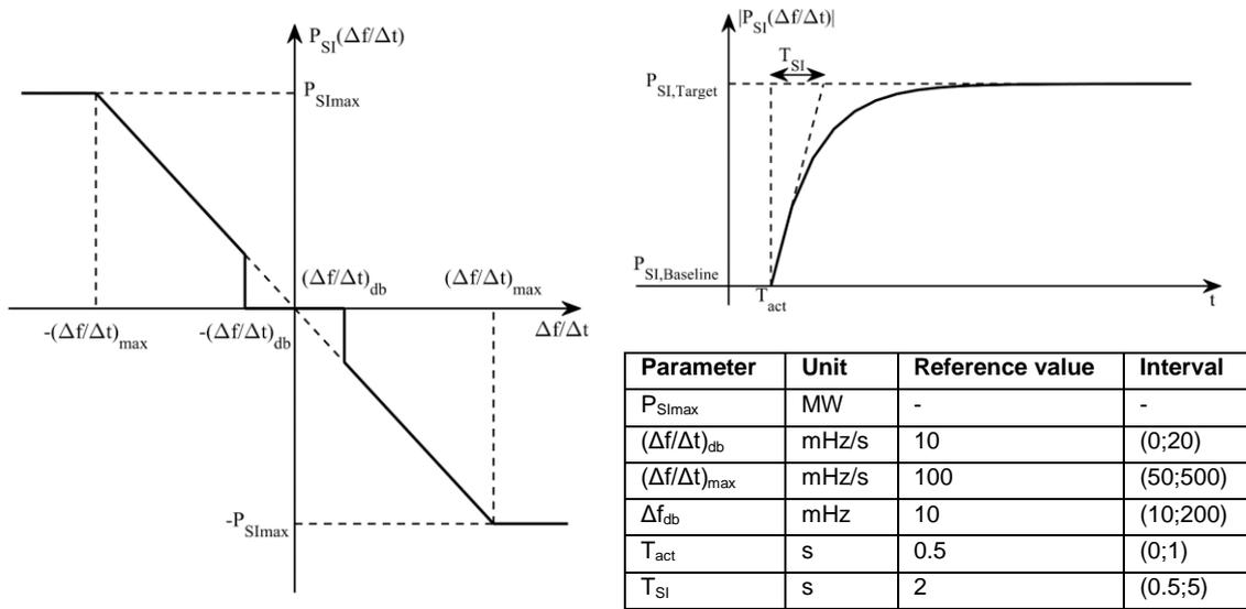
Figure 9: Frequency- and time-characteristic curves of SI
