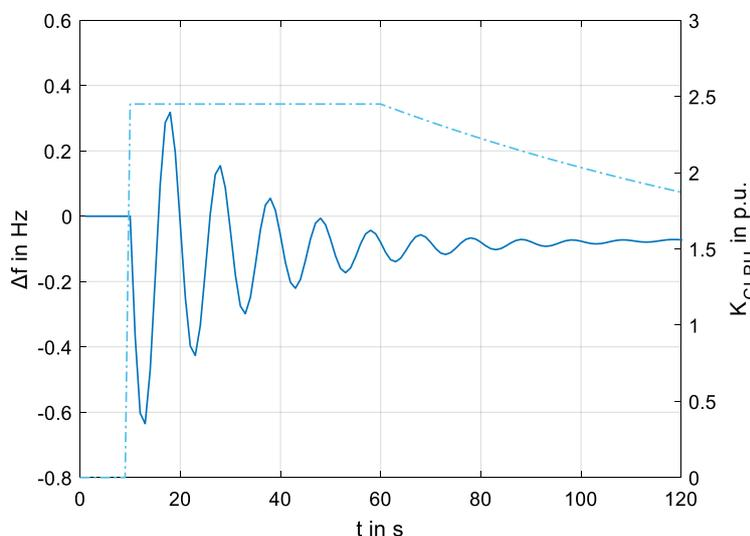
Figure 23: Frequency response of the system after load connection [13]
