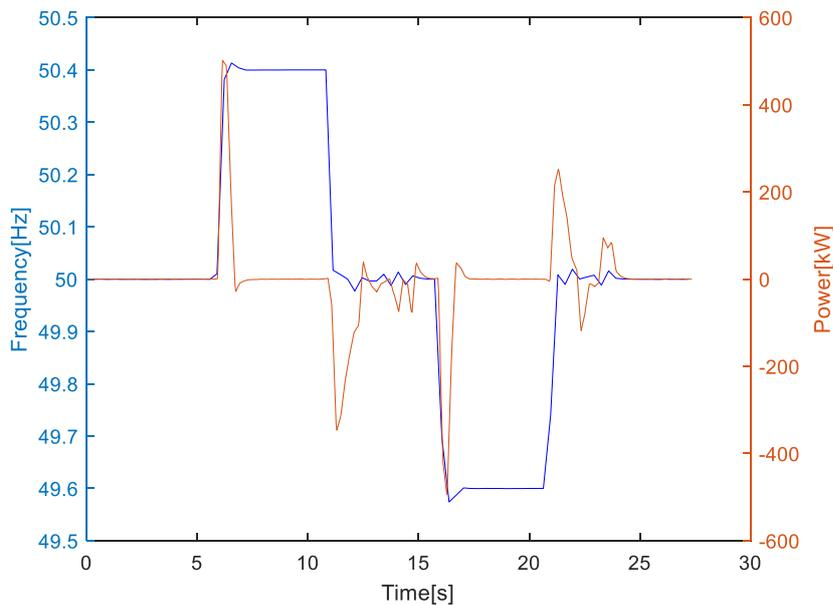
**Figure 38: SI function under a frequency step (test II)**
