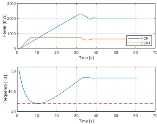
**Figure 80: Design hypothesis 2030 including FCR+ to keep the frequency  $\geq 49,2$  Hz**
