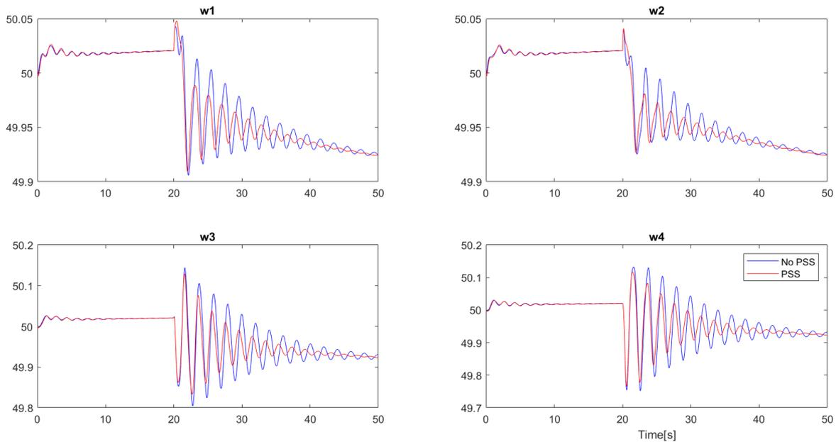
**Figure 51: Speed in all machines with and without PSS.**
