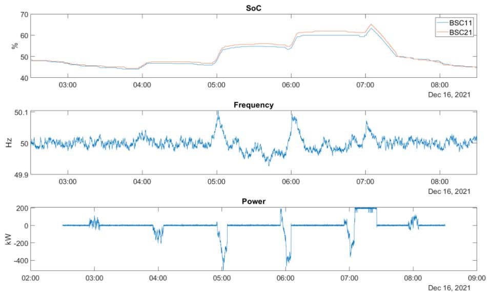
Figure 69: Behaviour of the DFD function and corresponding SoC evolution
