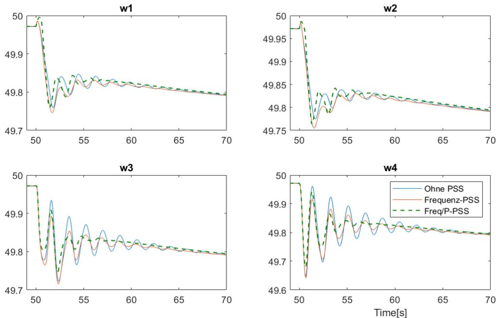
Figure 52: Frequency-only PSS vs Frequency & Power PSS
