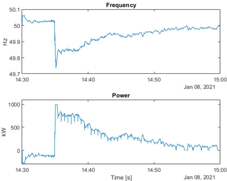
**Figure 53 - Behaviour of EFR for a grid split event (Thold = 30s)**
