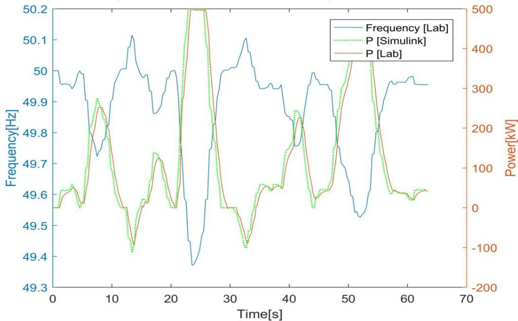
**Figure 33 - EFR response for continuous frequency deviations**
