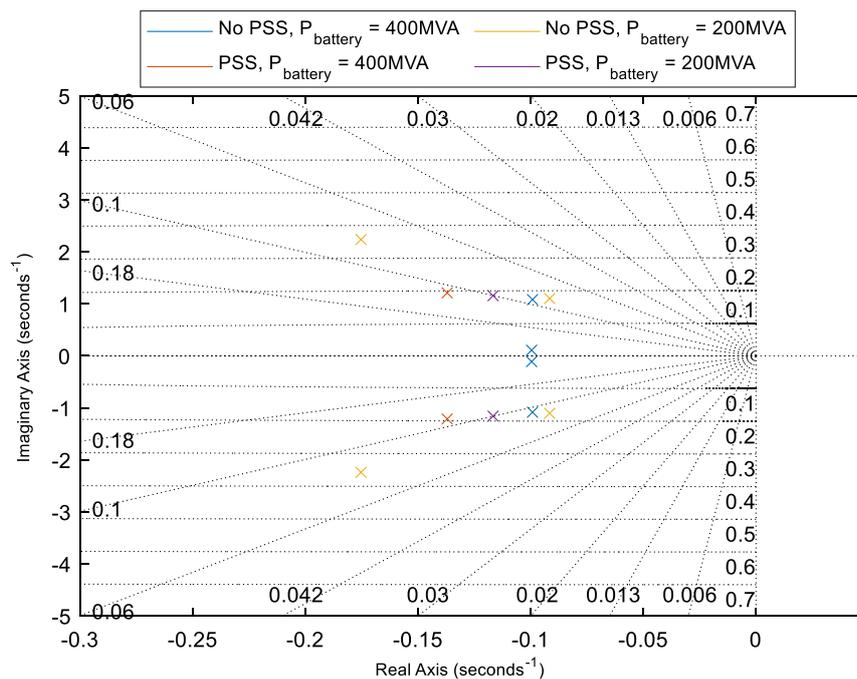
**Figure 17: Pole-zero diagram of inter-area oscillations under different battery capacities (oscillations checked from 161 to 180 s)**
