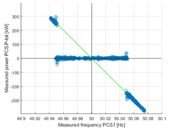
Figure 65: Specified static characteristic curve of FCR+ (left) and measured characteristic curve (right)
