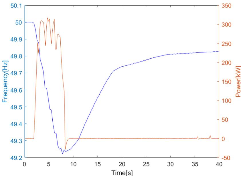
Figure 41: SI function under a slow frequency deviation (test II)
