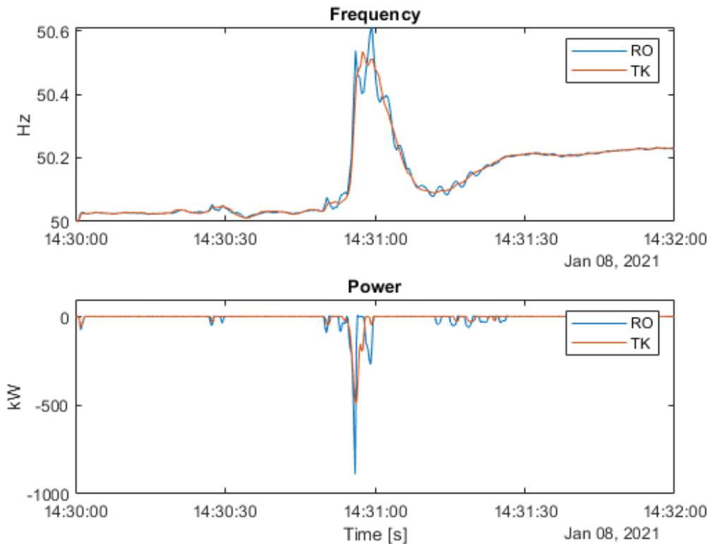
**Figure 56 - Behaviour of SI for a grid split event using different frequency measurements (East region)**
